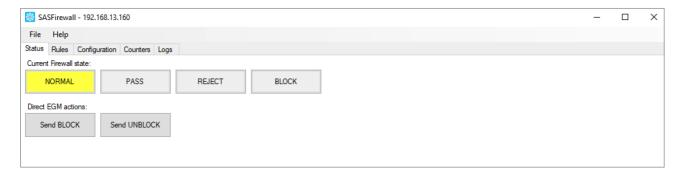
Screen for establishing pattern rules that match the SAS commands to execute the different actions as appropriate. (Pass – Reject – Block).
